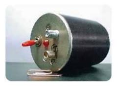
Waveguide Noise Source
