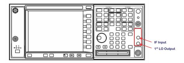
Figure 3: Diagram of Front Panel
