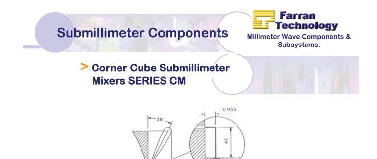
Figure 2. Corner Cube Mixer have 24° wide (at 10dB points) Gaussian beam at an angle of 28° to the vertical
